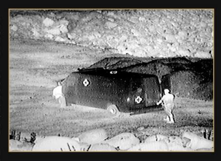
the shape of the insignia on the ThermoEmblem starts emitting broadband infrared radiation. The insignia stands out exceptionally from its surroundings when viewed with thermal imaging gear. There is a surface temperature difference of approximately 20°C (68°F) above ambient in any weather conditions. This enables friendly vehicles to be positively identified from a distance of several kilometres.
